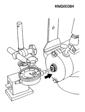
Checking and adjusting armature axial clearance
